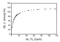
**Figure 4.** Magnetization (M) versus magnetic field/temperature (H/T) at ( $\blacksquare$ ) 200 K, (+) 250 K, and ( $\diamondsuit$ ) 290 K, after correcting for the temperature dependence of spontaneous magnetization ( $I_s/I_o$ ) for the nanometer iron colloid particles dispersed in a polyvinylpyrrolidone matrix
