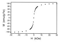
**Figure 3.** Magnetization hysteresis loops for the nanometer iron particles dispersed in a PVP matrix at 250 K: (+) magnetization data points; (■) demagnetization points. No hysteresis is observed and consequently the magnetization data points are overlapped by the demagnetization data.
